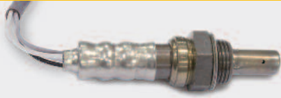
Automatic exhaust and combustion monitoring via lambda probe control
