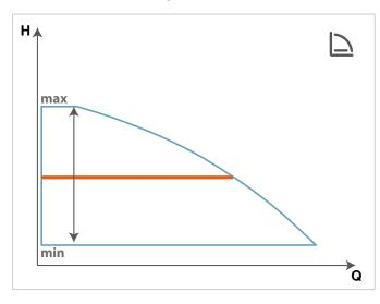
The circulator maintains a constant pressure level (head) upon the decreasing demand for heat from the system (reduced flow rate).
