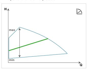
The innovative electronics of the circulator, developed in Taco Italia laboratories, proportionally reduces the pressure level (head) according to the reduction of the heat requested by the system (reduced flow). A proportional curve can be selected within the allowed flow rate range.
