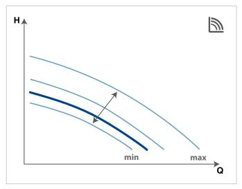
**ENERGY SAVING** features fixed speed adjustable operating curves by positioning the regulator at any point between the Min and Max positions; as a result it is possible to meet any installation requirements (from the single pipe, to the most modern and sophisticated systems) and ensure optimum performance.
