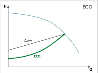
In **ECO mode** the circulator consumes even less energy, resulting in greater overall energy savings. In **ECO mode** the circulator creates a quadratic type of adjustment curve.
