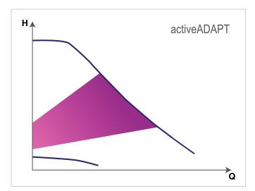
The **activeADAPT** mode enables the circulator to actively adapt its performance to the demands of the system during short control intervals inside a defined control area. If the system requirements suddenly change, the circulator will automatically find the perfect curve.
